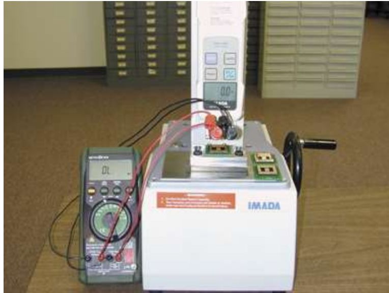
Figure 3: Insertion/Extraction test setup
