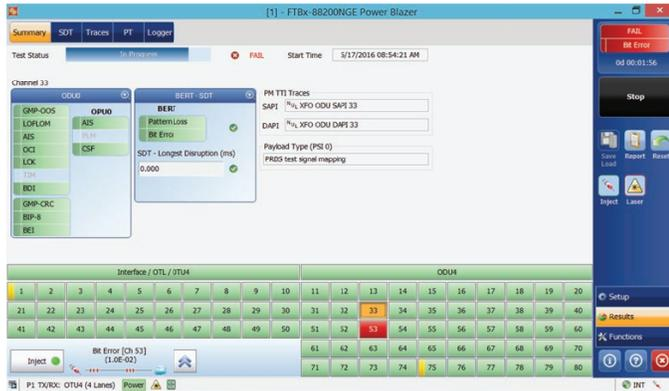
Figure 16: FTBx-88200NGE - Summarized alarm and error indication for all 80 ODU0 channels composing an OTU4 signal
