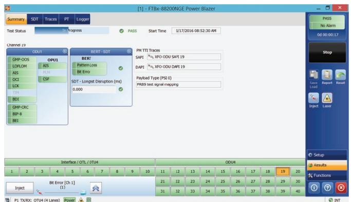
Figure 14: FTBx-88200NGE - Summary view of all channels: OTU4/ODU4/ODU1 mapping
