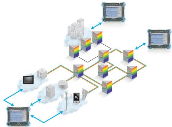
Figure 3: Mesh configuration
