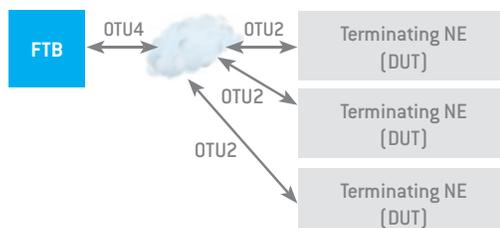
The Multichannel OTN Test Application supports single stage multiplexing (Figure 5): ODU0 > ODU4, ODU1 > ODU4, ODU2 > ODU4, ODU3 > ODU4 channels. The technician can specifically select the mapping to be exercised among the following multiplexing options:
