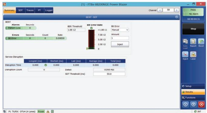
Figure 19: FTBx-88200NGE - Detailed BER results per channel
