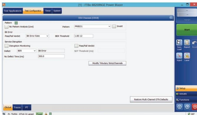
Figure 17: FTBx-88200NGE - BER test configuration
