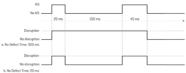
Figure 22: Service disruption scenarios based on different No Defect Time configurations
