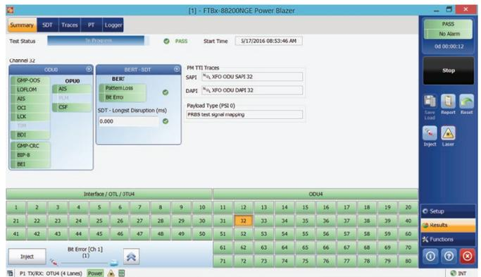
Figure 15: FTBx-88200NGE - Summary view of all channels: OTU4/ODU4/ODU0 mapping
