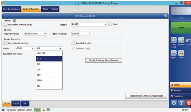
Figure 21: FTBx-88200NGE - Defect selection for SDT measurement
