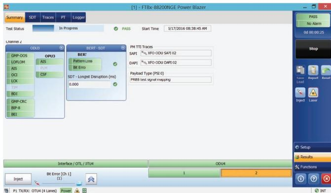
Figure 12: FTBx-88200NGE - Summary view of all channels: OTU4/ODU4/ODU3 mapping
