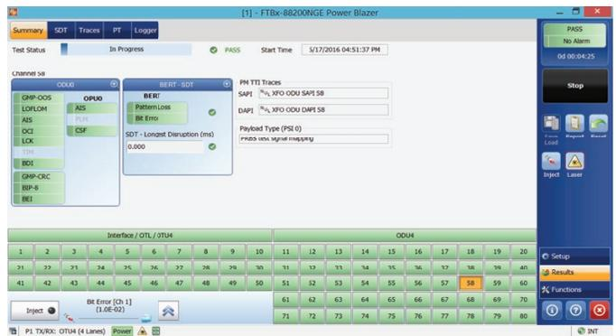
Figure 18: FTBx-88200NGE - Simultaneous monitoring of all channels
