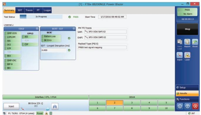
Figure 13: FTBx-88200NGE - Summary view of all channels: OTU4/ODU4/ODU2 mapping
